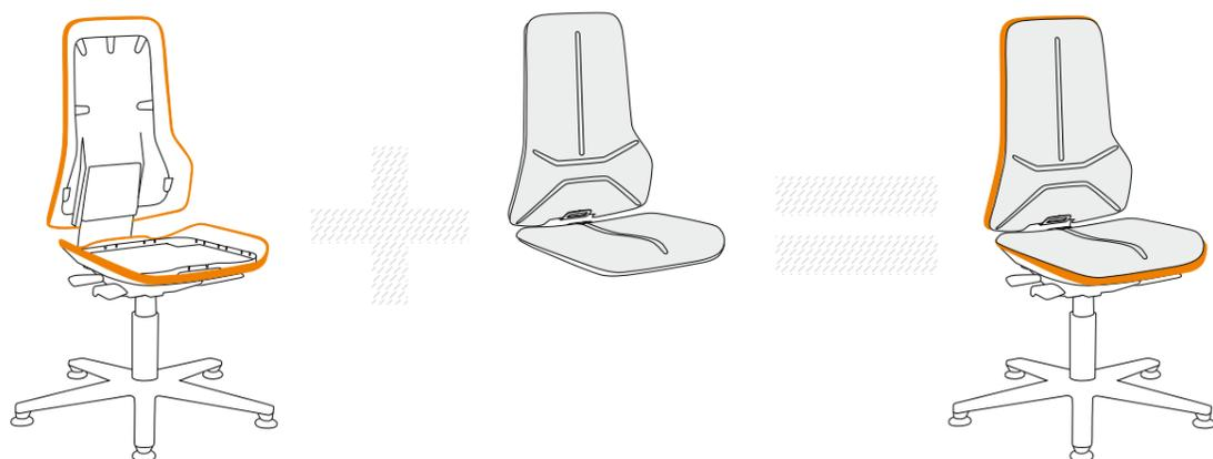
Neon consists of two elements: the chair element with base and mechanism and the upholstery element. Both elements can be configured independently and are freely combinable. This offers many advantages:
